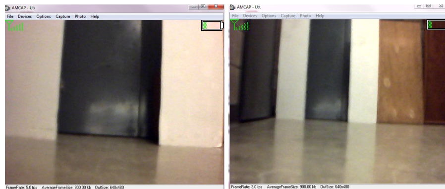
Figure 2.6 Distorted display with true distance being 5 feet (left: true distance; right: displayed distance)
